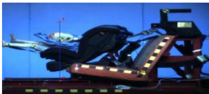
Figure 4 high-speed camera measured displacement of p3 dummy head
